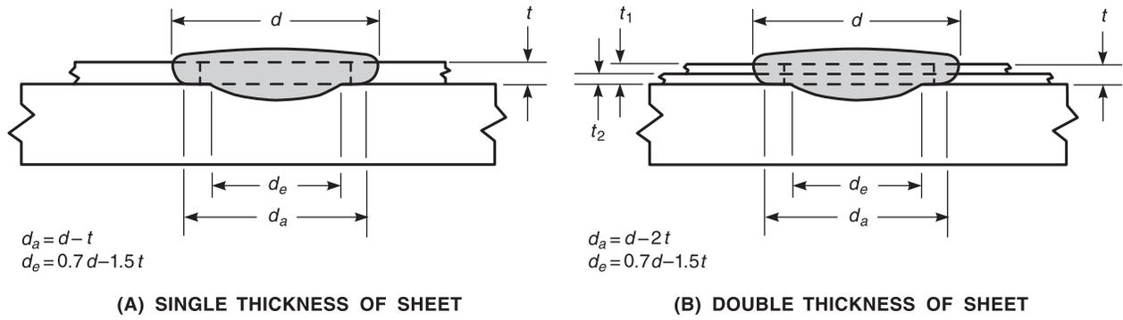
Figure 2.6—Arc Plug Welds (see 2.2.6)
