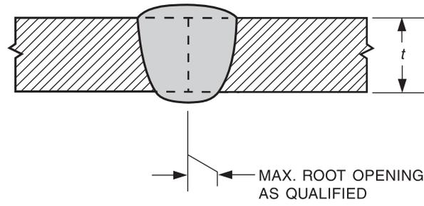
Note: The groove weld size equals the thickness  $t$ .
