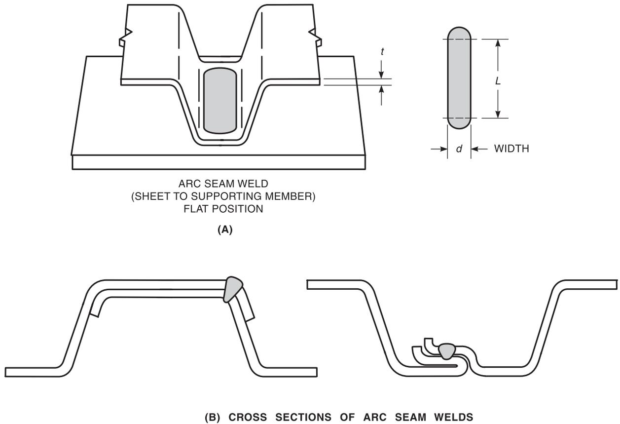
Figure 2.5—Arc Seam Welds (see 2.2.5)
