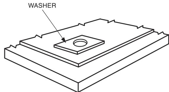
**Figure 2.11C—Typical Weld Washer (see 2.3.5.3)**
