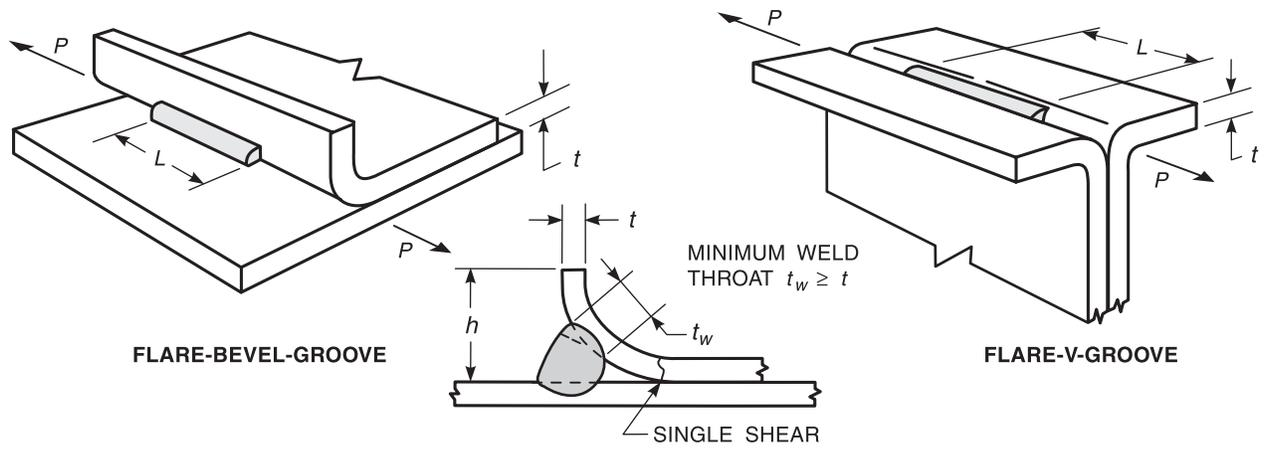
Figure 2.3B—Single-Shear in Flare-Groove Welds [see 2.2.3(2)]
