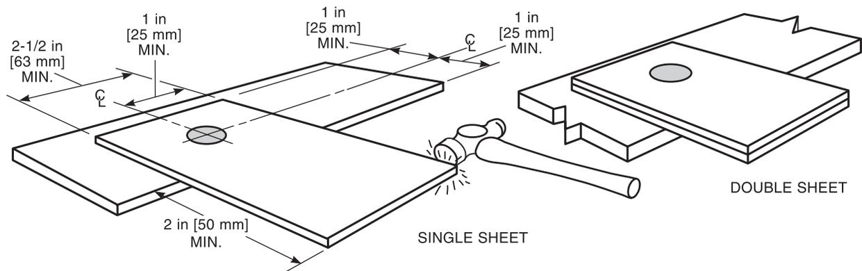
**Figure 4.4—Test for Arc Spot Welds [see 4.6.4.2(1)]**
