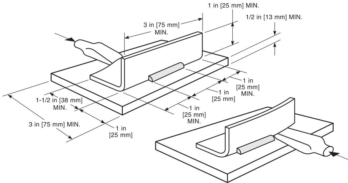
**Figure 4.3B—Test for Sheet to Supporting Structural Member Flare-Bevel-Groove Welds [see 4.6.3.2(1)(b)]**
