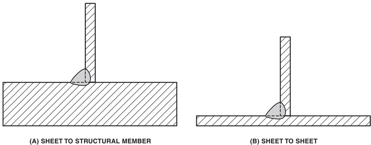
Figure 2.8—Fillet Welds in T-Joints (see 2.3.3.2)
