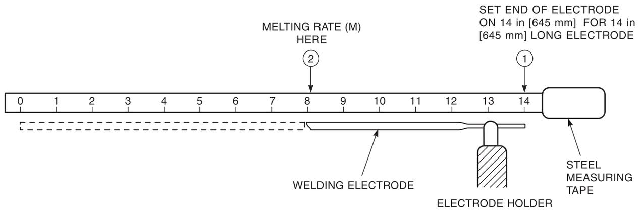
**Figure C-4.1—Melting Rate Measurement Illustrated**
