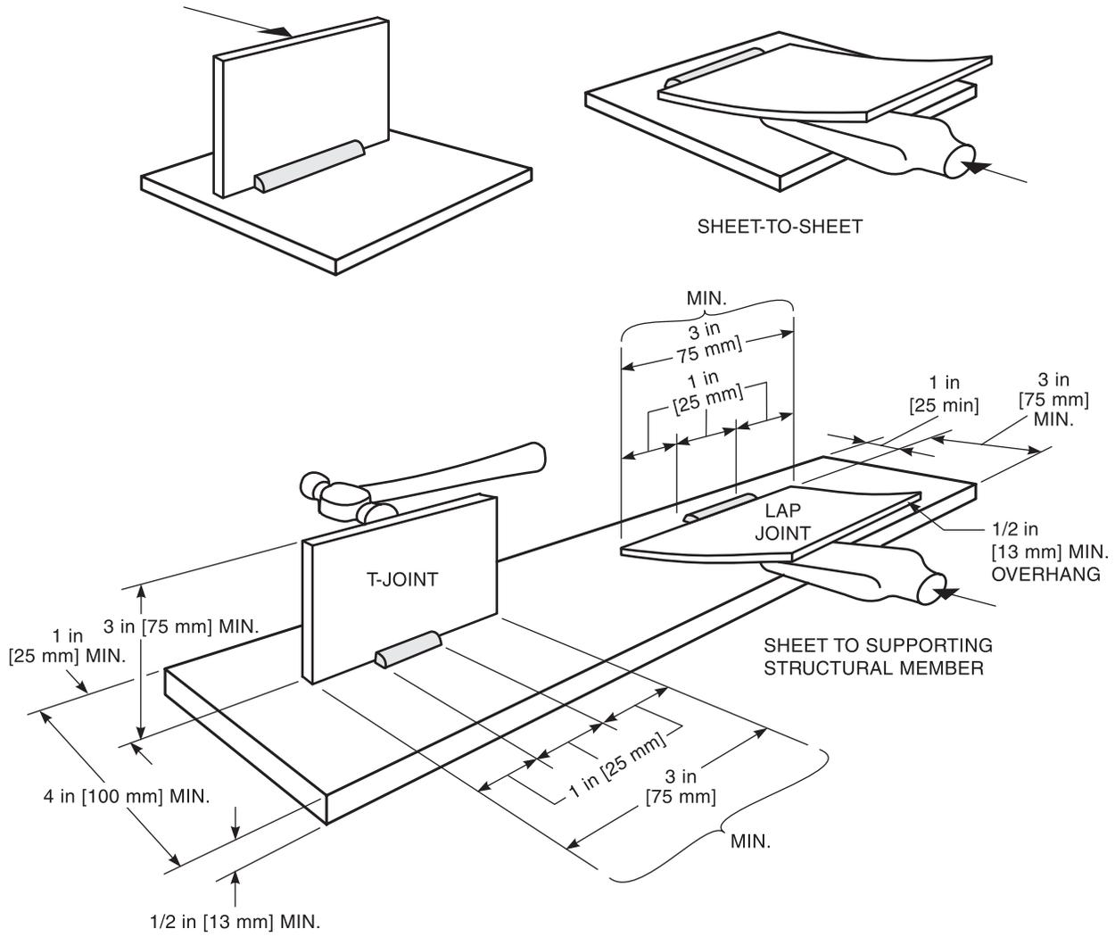
**Figure 4.2A—Test for Fillet Welds [see 4.6.2.2(1)]**
