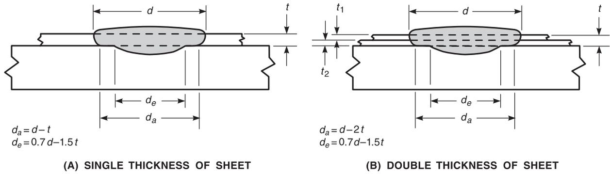
Figure 2.4—Arc Spot Welds (see 2.2.4)
