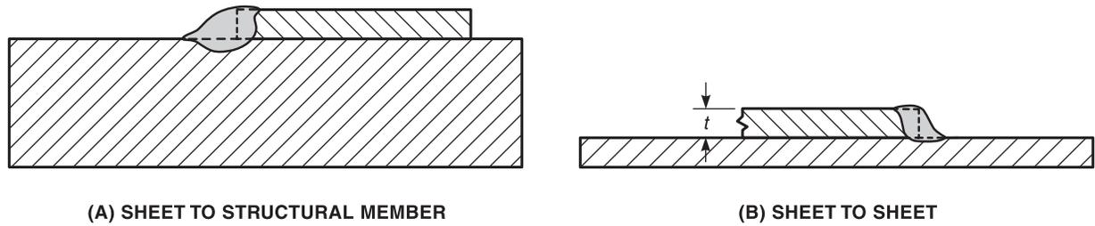
Figure 2.7—Fillet Welds in Lap Joints (see 2.3.3.2)
