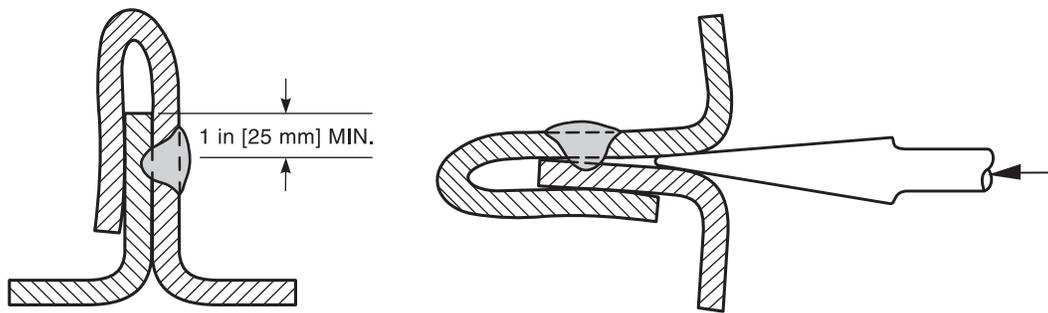
**Figure 4.5B—Test for Sheet to Sheet Arc Seam Welds [see 4.6.5.2(2)]**
