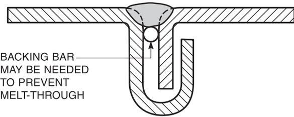
**Figure 2.10—Single-Flare-V-Groove Weld (see 2.3.4.2)**
