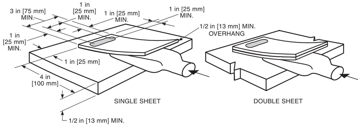
**Figure 4.5A—Test for Sheet to Supporting Structural Member Arc Seam Welds [see 4.6.5.2(1)]**
