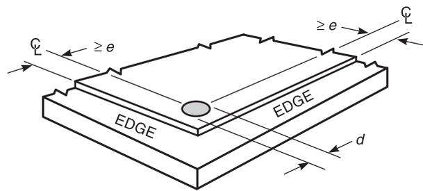
**Figure 2.13B—Edge Distances for Arc Plug Welds (see 2.3.7.3)**
