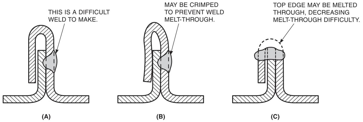
**Figure 2.12—Arc Seam Welds Along Standing Rib (see 2.2.5)**
