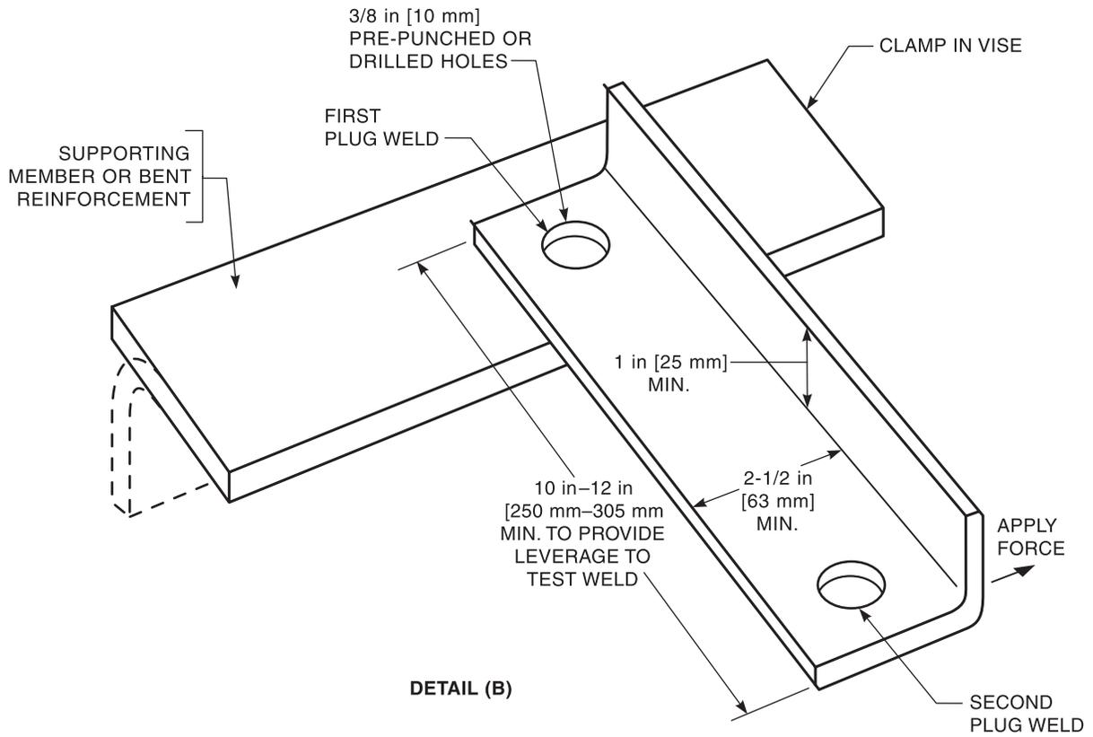
**Figure 4.6 (Continued)—Test for Arc Plug Welds [see 4.6.2.2(1)]**
