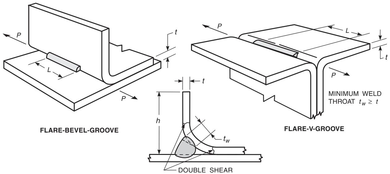
Figure 2.3C—Double-Shear in Flare-Groove Welds [see 2.2.3(2)]
