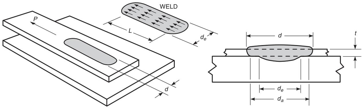
**Figure C-2.4—Arc Seam Weld in a Supporting Plate**
