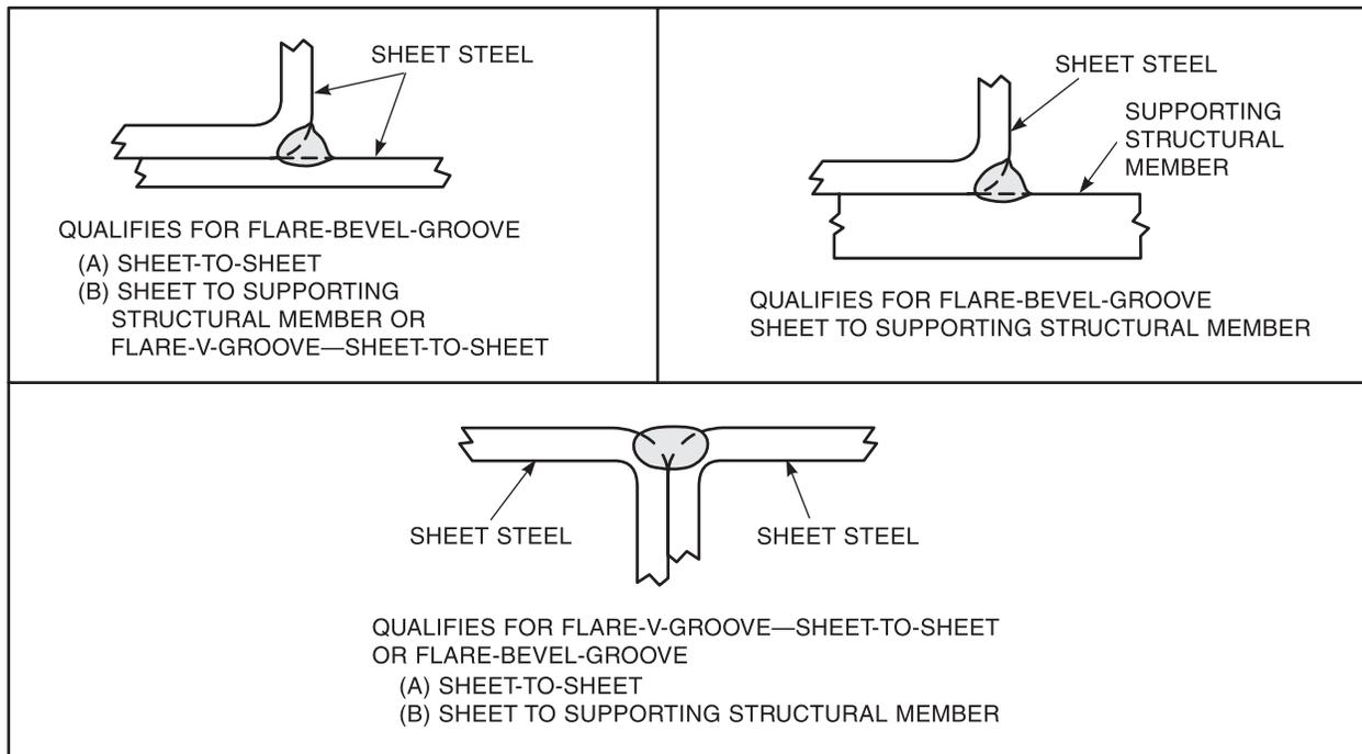
**Figure 4.3D—Extent of Validity of Flare-Groove Weld Qualifications (see 4.6.3.3)**
