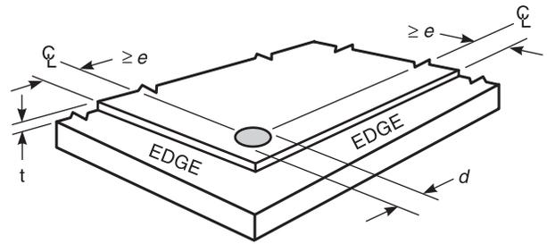
**Figure 2.11A—Edge Distances for Arc Spot Welds (see 2.3.5.2)**
