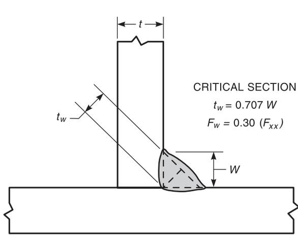
**Figure C-2.1—Allowable Stress for Fillet Welds**
