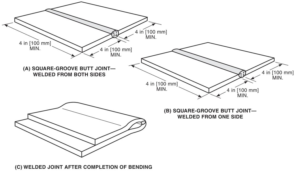
**Figure 4.1—Test for Square-Groove Welds in Butt Joints [see 4.6.1.2(1)]**
