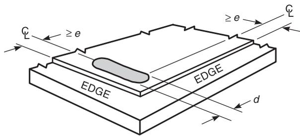
**Figure 2.13A—Edge Distances for Arc Seam Welds (see 2.3.6.3)**
