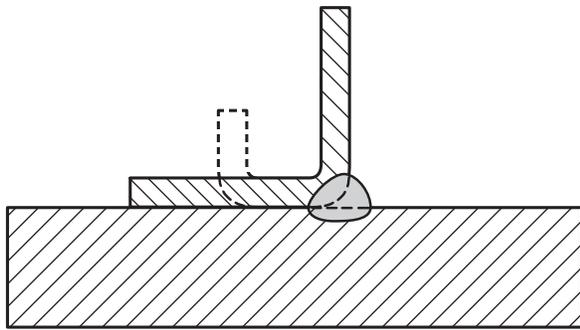
**Figure 2.9—Single-Flare-Bevel-Groove Weld (see 2.3.4.1)**
