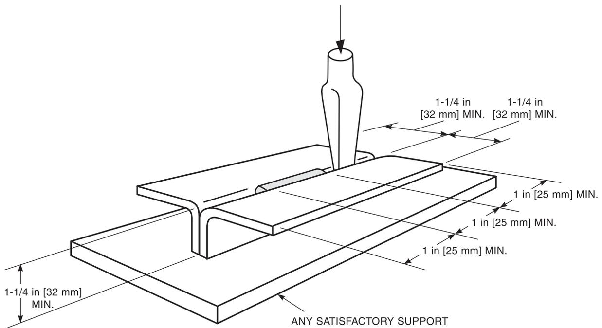
**Figure 4.3C—Test for Flare-V-Groove Welds [see 4.6.3.2(2)(b)]**
