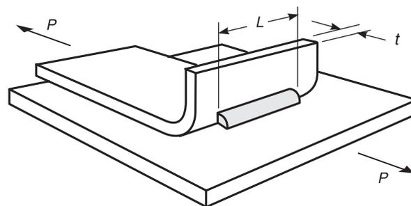
**Figure 2.3A—Single-Flare-Bevel-Groove Weld [see 2.2.3(1)]**
